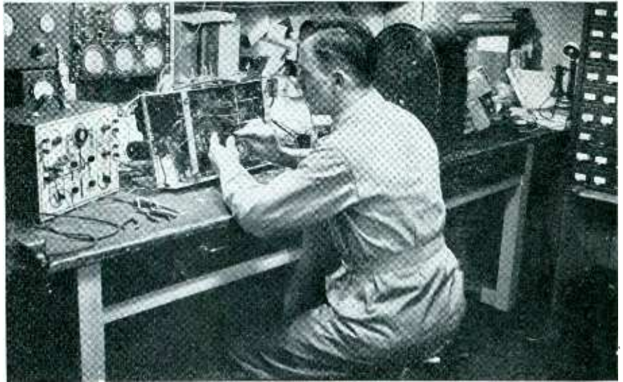
PEAKING—Cliff Weidenbauer, Jones and Polk, Detroit, goes further; he tunes 'em right on the button with an oscillograph and wobulator.
